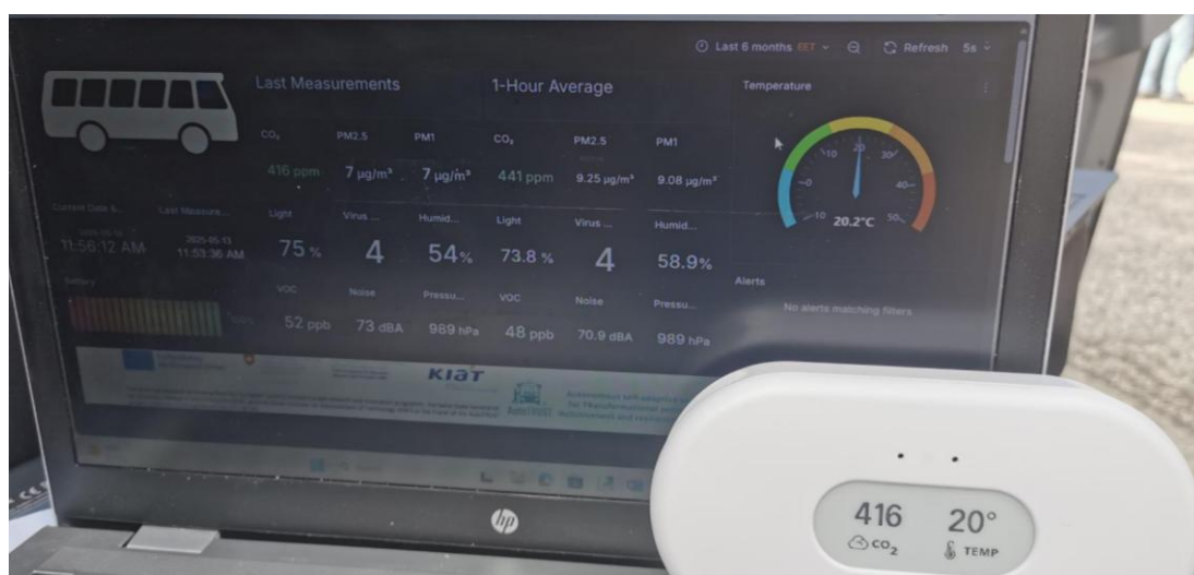
Figure 31: Example of the in-vehicle environment stationary sensor and visualization interface.
